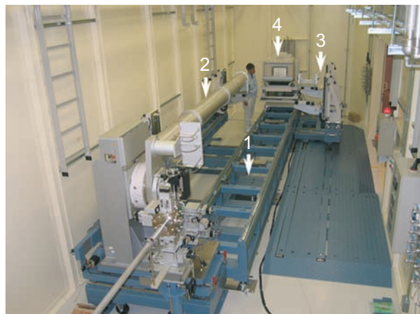
Fig. 2. Photograph of the SAXS camera in BL08B2 experimental hutch 2: (1) guide rail, (2) long vacuum tube (6 m camera length), (3) carrier stage for middle- or short-length vacuum path, (4) SAXS detector.
