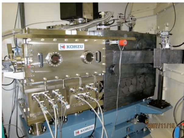
Fig. 2. Installed diamond monochromator in the first optical hutch.
