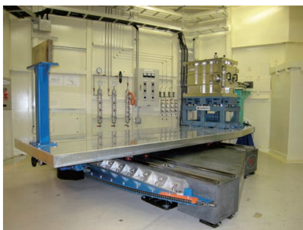
Fig. 3. High-resolution monochromator installed on the rotational platform in the experimental hutch.
