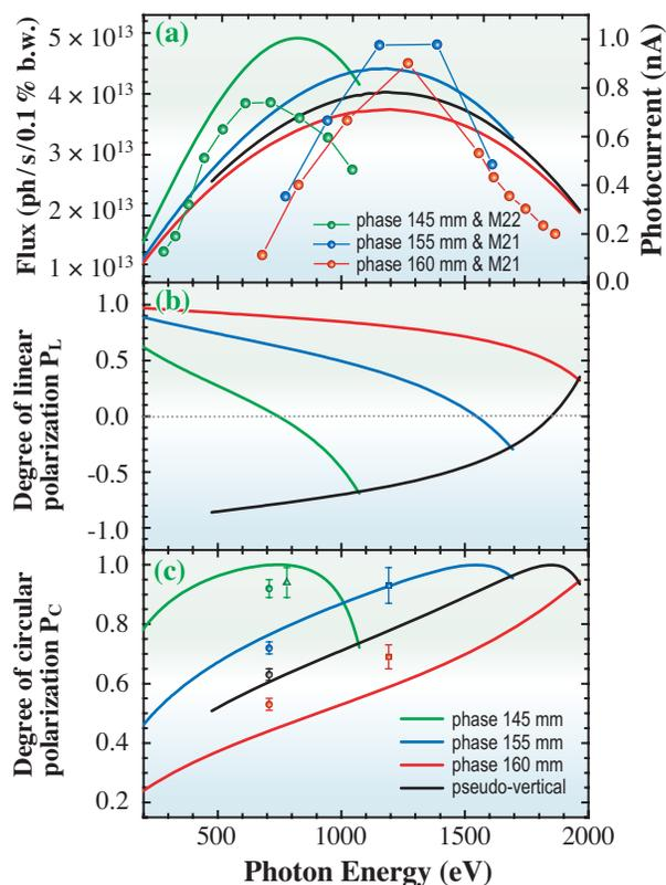
Fig. 1. Calculated and measured characteristic features of the SX beam from ID17.
