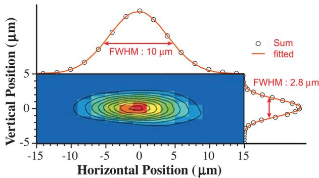
Fig. 3. Measured beam profile at E2a station.
