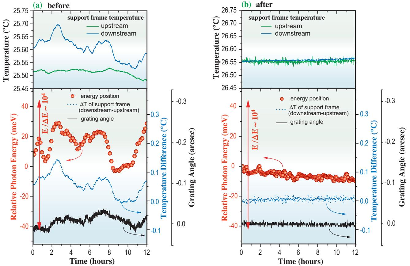
Fig. 2. Relative photon energy (red circles), grating rotation angle (black line), support frame temperature of the upstream (green line) and downstream (blue line), and the temperature difference of the support frame (blue dotted line) measured at 867 eV before (a) and after (b) installation of the TSS.
