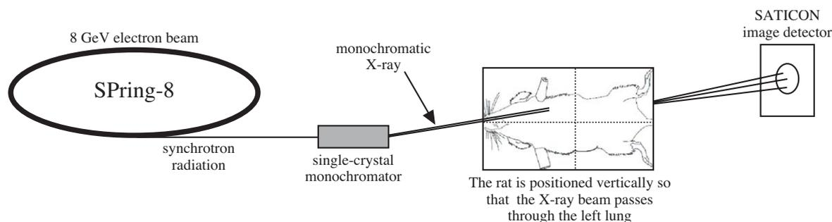
Fig. 1. A simplified schematic diagram showing the experimental set-up for pulmonary microangiography in a closed-chest rat model using SR.
