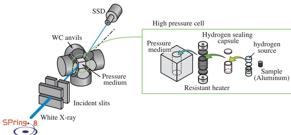
Fig. 1. Schematic of *in situ* X-ray diffraction measurement system and high-pressure cell.
