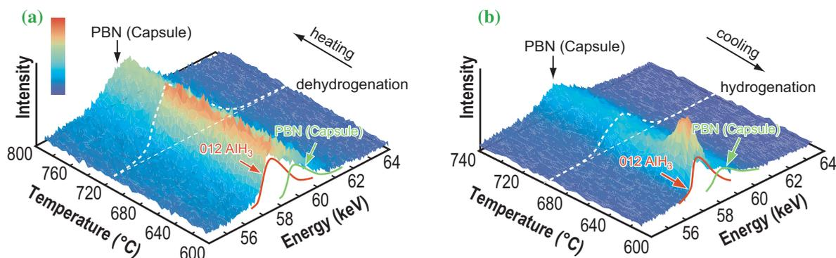
Fig. 2. Temperature variation of X-ray diffraction profiles taken at 10.0 GPa during (a) heating and (b) cooling.
