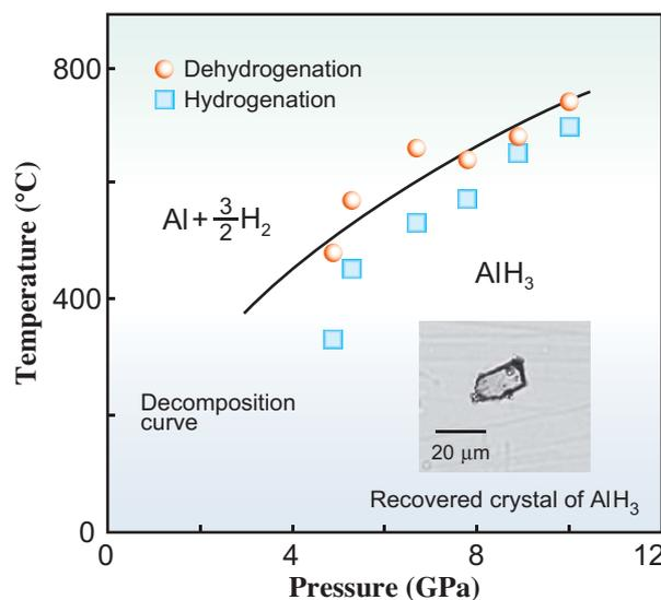
Fig. 3. Hydrogenation and dehydrogenation pressure-temperature conditions determined by *in situ* X-ray diffraction measurements. Inset shows a micrograph of a recovered AlH<sub>3</sub> crystal.
