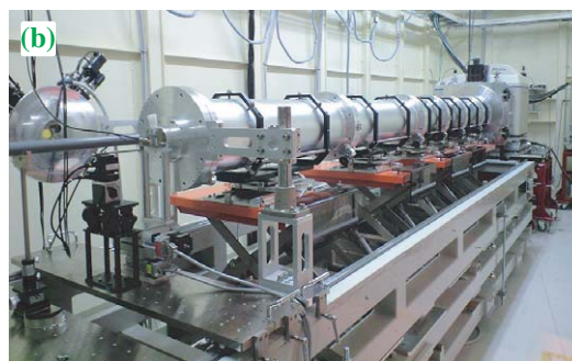
Fig. 2. Photographs settings at BL40B2 of camera lengths of (a) 0.25 m and (b) 4 m.
