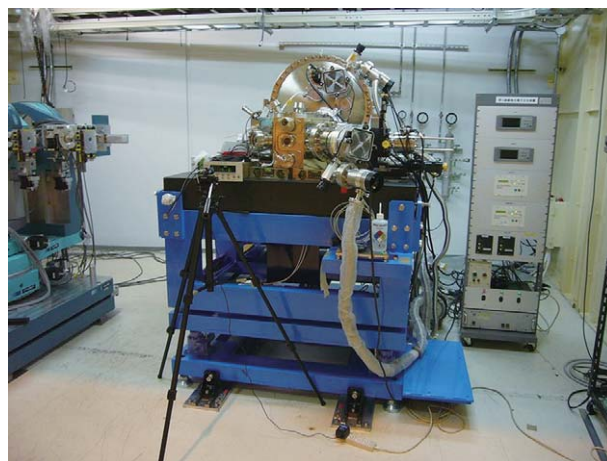
Fig. 3. The device for hard X-ray photoemission spectroscopy.
