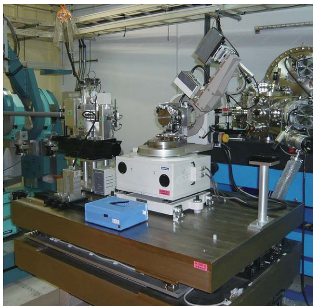
Fig. 2. X-ray diffractometer specialized for the thin film analysis (ATX-G).
