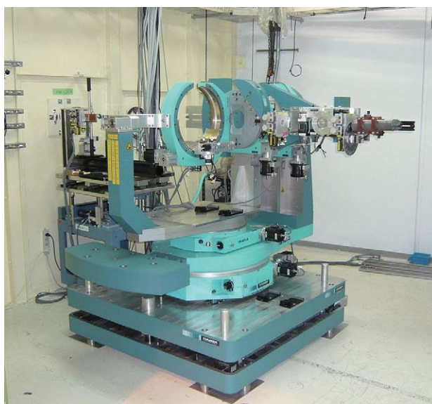
Fig. 1. Multi-axis X-ray diffractometer.
