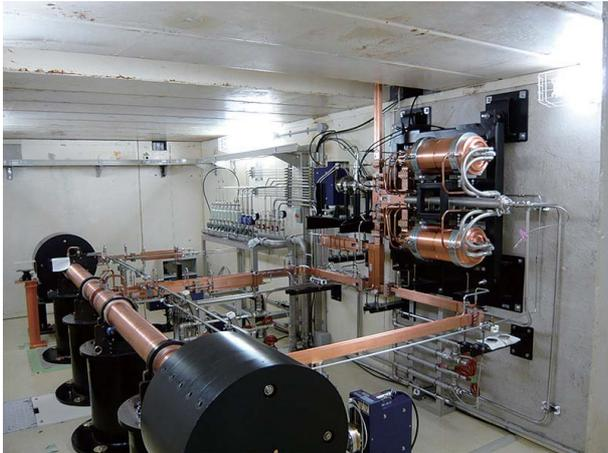
Fig. 2. Test bunker for high-power rf components.
