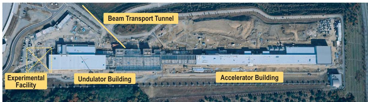
Fig. 10. Aerial photograph of XFEL construction site taken in November 2008.
