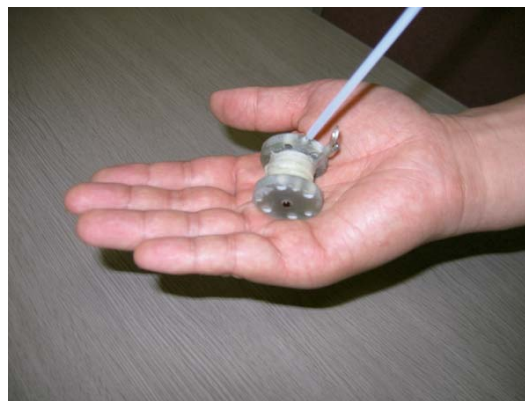
Fig. 1. Photograph of solenoid miniature magnet for XMCD measurement. The inner diameter is 3 mm. Maximum fields of up to 50 T can be generated. For a repetition of more than 300 shots, the maximum field is limited to 40 T for the XMCD experiment.
