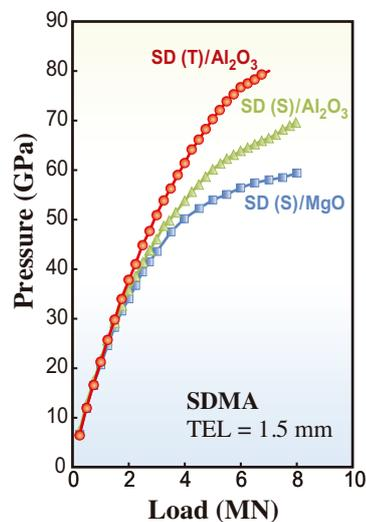
Fig. 1. Pressures generated using SDMA. Two kinds of sintered diamond, Al<sub>2</sub>O<sub>3</sub> and MgO ceramics, were tested as the anvil and pressure medium, respectively.
