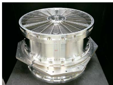
Fig. 1. Hard X-ray mirror on board SUMIT balloon experiment. 199 pairs of conically approximated Wolter-I optics are nested coaxially. Aperture diameter, mirror length, and focal length are 40 cm, 26 cm, and 8 m, respectively.
