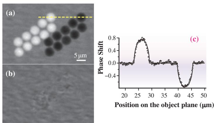
Fig. 2. (a) Enlarged phase-difference image of the PS spheres (gray scale,  $-0.3\pi - 0.3\pi$ ). (b) Absorption image of the same area as (a) obtained by simply removing the grating. (c) Section profile along the dashed line in (a). [4]
