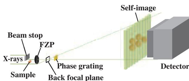
Fig. 1. Setup of phase-difference X-ray microscopy with a transmission phase grating (side view). [3]
