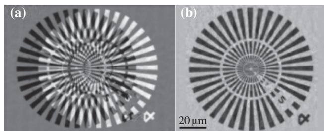
Fig. 3. (a) Differential phase image of a  $1\text{-}\mu\text{m}$ -thick tantalum Siemens star chart and (b) its phase image retrieved from (a). [4]
