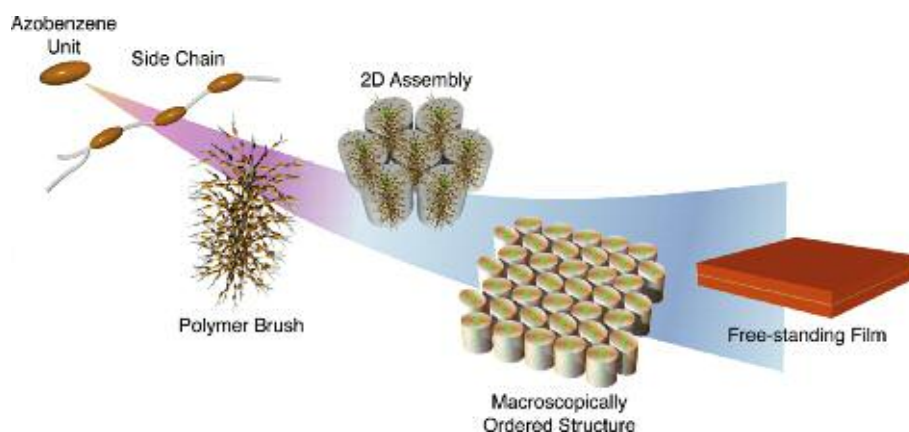
Fig. 3. Schematic illustration of 3D molecular order in hot-pressed polymer brush film.
