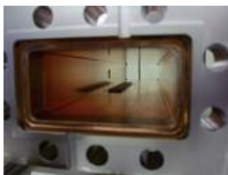
Fig. 11. (a) Prototype isolator composed of waveguide and permanent magnets. (b) Rectangular ferrite plate bonded to internal surface of waveguide.
