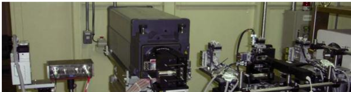
Fig. 2. Photograph of sub-10 nm focusing system installed in the 1-km-long beamline (BL29XUL).
