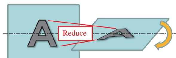
Fig. 1. Illustration of size reduction effect in glancing view.
