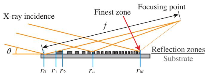
Fig. 2. Schematic of the total reflection zone plate.
