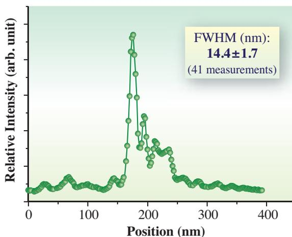
Fig. 3. Measured intensity distribution of line focus obtained with the TRZP.
