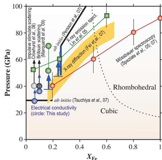
Fig. 3. Spin transition pressures as a function of  $X_{\text{Fe}}$  in the  $(\text{Mg}_{1-x},\text{Fe}_x)\text{O}$  solid solution at 300 K. Blue solid circles indicate the spin transition pressure determined in this study and the arrow represents the mixed spin state. Blue horizontal bars indicate the minimum transition pressure. The other symbols represent the spin transition pressure or crossover predicted by different experimental techniques (modified after [2]).
