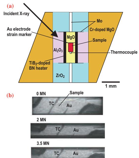
Fig. 1. (a) Schematic cross section of the cell assembly used in our experimental runs. (b) X-ray radiography images of the sample and the thermocouple through the TiB<sub>2</sub> heater at various press loads (in MN).
