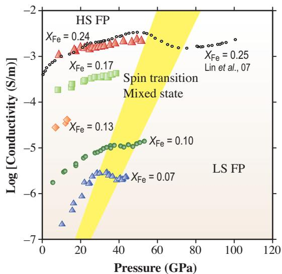
Fig. 2. Electrical conductivities of  $(\text{Mg}_{1-x},\text{Fe}_x)\text{O}$  as a function of pressure at a constant temperature of 300 K. At low pressures, the conductivity constantly increases but the conductivity of FP with relatively lower  $X_{\text{Fe}}$  drops or becomes constant from 30 to 45 GPa. Large symbols denote the data obtained in this study. Small open symbols denote the electrical conductivity of  $(\text{Mg}_{0.75},\text{Fe}_{0.25})\text{O}$  obtained from the DAC study.
