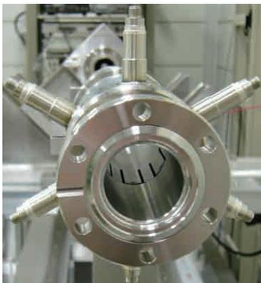
Fig. 9. Six-electrode BPM with circular cross section.
