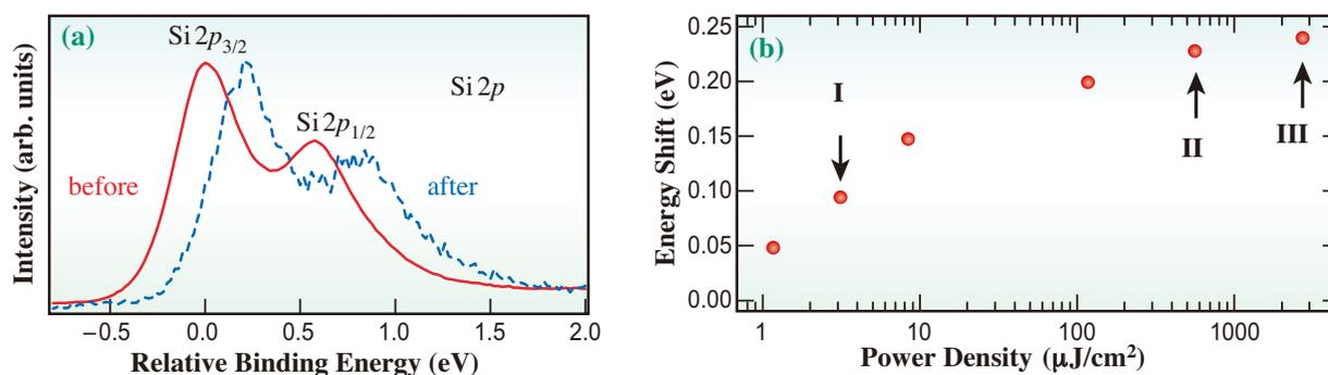
**Fig. 1.** (a) Si 2*p* core-level spectra ( $h\nu = 253$  eV) before and after the laser irradiation are shown as solid (red) and dashed (blue) lines, respectively. The power density of the pump laser ( $h\nu = 1.51$  eV) was  $2700 \mu\text{J}/\text{cm}^2/\text{pulse}$ . (b) Energy shift of Si 2*p* spectra, measured at different power densities or photon densities. The delay time between the pump laser and probe synchrotron pulses was set at 1 ns.
