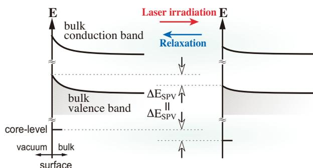
Fig. 2. Schematic of photovoltage effect at semiconductor surface. Bulk bands bend in energy as they approach a surface (surface band bending effect). Energy shift ( $\Delta E_{SPV}$ ) of the bulk band at the surface, induced by laser irradiation, corresponds to that of the core level.
