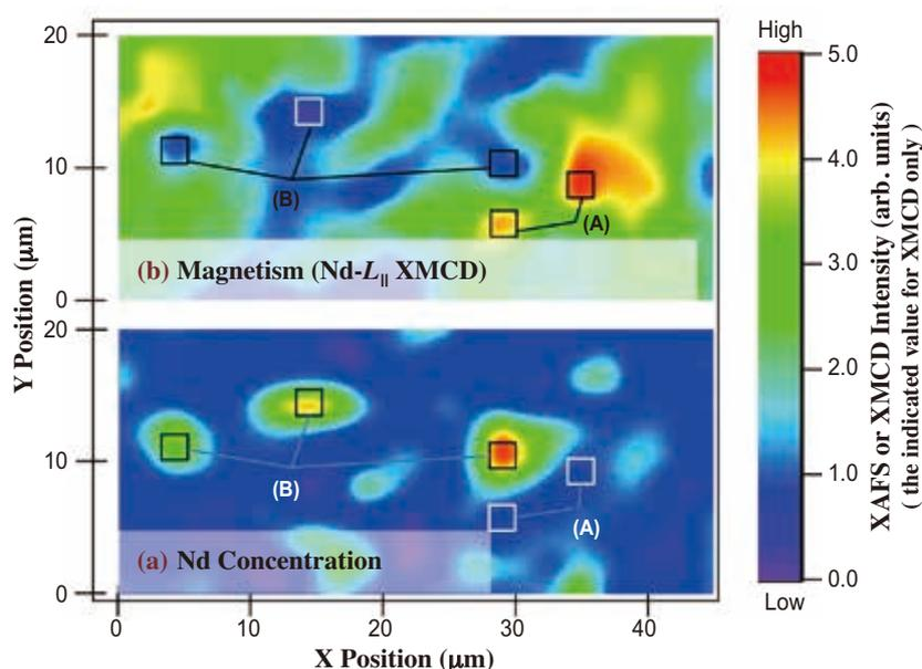
Fig. 3. Experimental results obtained using our magnetic/elemental microscope at BL16XU. (a) Elemental map for Nd concentration obtained by measuring Nd- $L_{\alpha}$  fluorescence and (b) HXMCD signal map of Nd- $L_{\alpha}$  XMCD. Area (A) is a crystalline  $Nd_2Fe_{14}B$  alloy and area (B) consists of Nd-rich paramagnetic precipitates.
