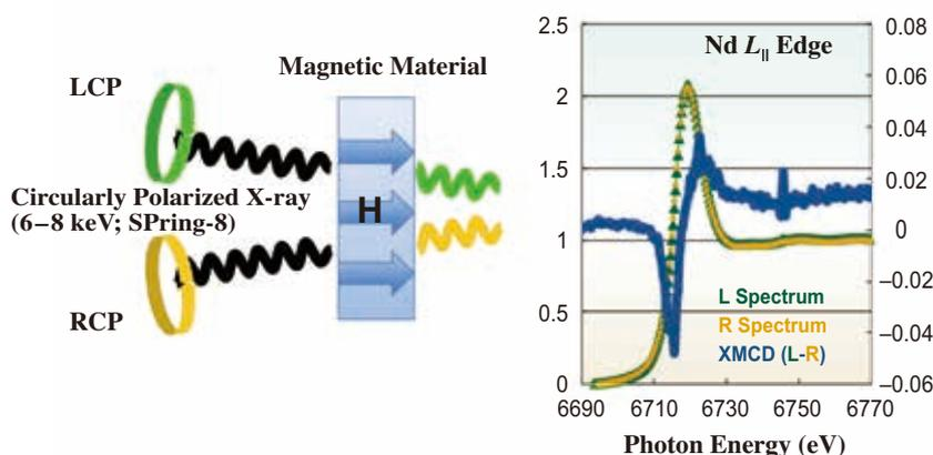
Fig. 2. (Left) Conceptual drawing of (H)XMCD measurement. The arrows in the magnetic material indicate the direction of magnetization. The X-ray absorption probability depends on the relation (parallel/antiparallel) between the X-ray helicity (LCP/RCP) and magnetized direction. (Right) Example of Nd  $L_{II}$  HXMCD spectrum derived from two spin-dependent spectra.
