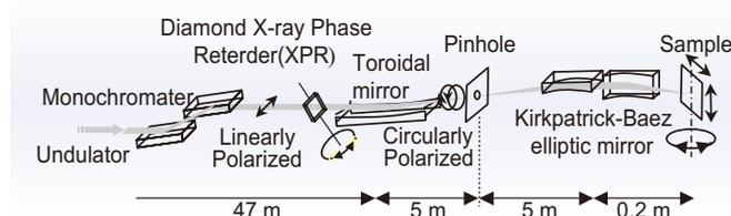
Fig. 1. Schematic drawing of our magnetic/elemental microscope system at BL16XU.
