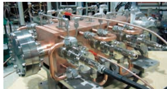
Fig. 6. New high efficiency longitudinal energy kicker (3 kicker cells inside).
