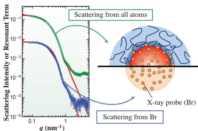
Fig. 3. SAXS and ASAXS profiles from TBC-incorporated polymeric micelles and their interpretation, showing the TBC distribution in the micelle. The red region represents the hydrophobic core, the blue lines represent PEG chains, and the orange polygons represent TBC.
