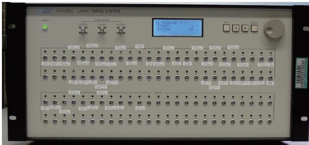
Fig. 13. Prototype of the trigger timing circuit with an FPGA. It has 50 NIM inputs, 50 NIM outputs, and 3 clock inputs. Half of the current timing system is programmed in the FPGA.
