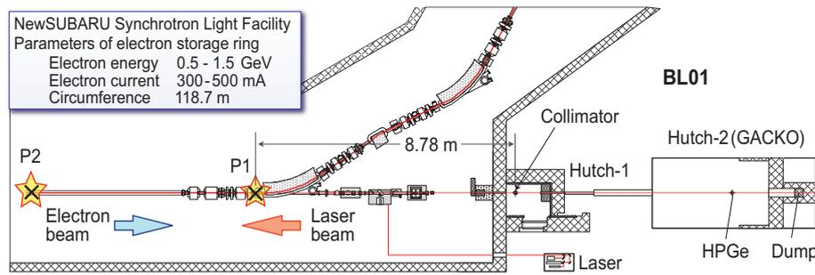
Fig. 3. Two  $\gamma$ -ray irradiation hutches are shown. Layout of laser Compton scattering  $\gamma$ -ray beam source in NewSUBARU BL01. Two collision points and two  $\gamma$ -ray irradiation hutches are shown.
