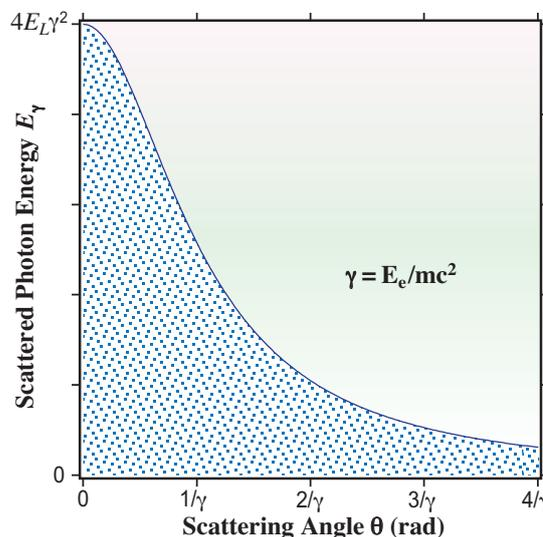
Fig. 2. Dependence of the  $\gamma$ -ray photon energy on the scattering angle  $\theta$ .
