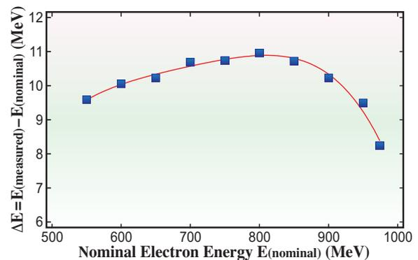
Fig. 4. The difference  $\Delta E$  of the calibrated energy  $E(\text{measured})$  from the nominal energy  $E(\text{nominal})$  of the electron beams,  $\Delta E = E(\text{measured}) - E(\text{nominal})$ , at the NewSUBARU storage ring.
