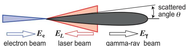
Fig. 1. Schematic of laser Compton scattering  $\gamma$ -ray generation at head-on collision.
