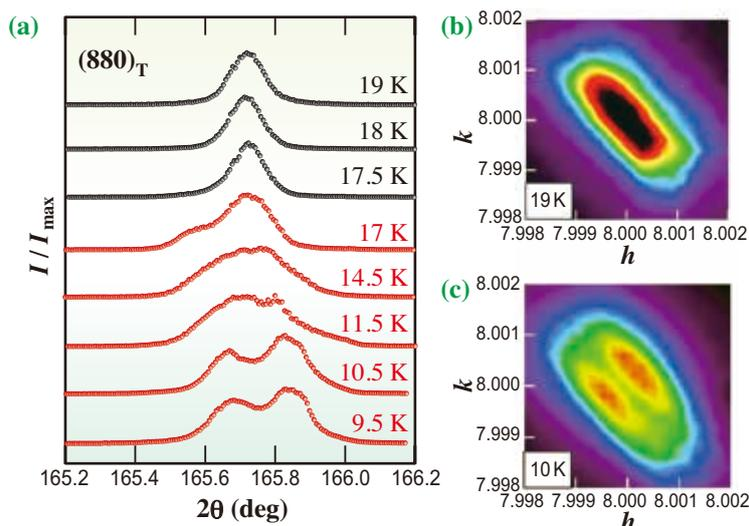
Fig. 2. (a) Temperature dependence of the Bragg peak  $(880)_T$  in an ultraclean single crystal of  $URu_2Si_2$ . Each curve is shifted vertically for clarity. Below the hidden order transition at  $T_{HO} = 17.5$  K, clear splitting of the Bragg peak is observed. (b) Two-dimensional intensity plot in the  $(hk0)$  plane near the  $(880)_T$  Bragg peak at 19 K (above  $T_{HO}$ ). (c) Similar data for 10 K (below  $T_{HO}$ ).
