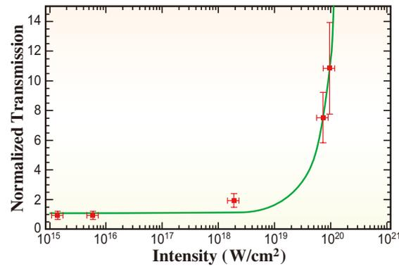
Fig. 2. Transmission normalized at the cold condition is plotted as a function of intensity at  $h\nu = 7.130$  eV for 20- $\mu\text{m}$ -thick iron foil. The square dots show the experimental results, while the green lines are simulated curves with core-hole lifetimes of 2 fs.
