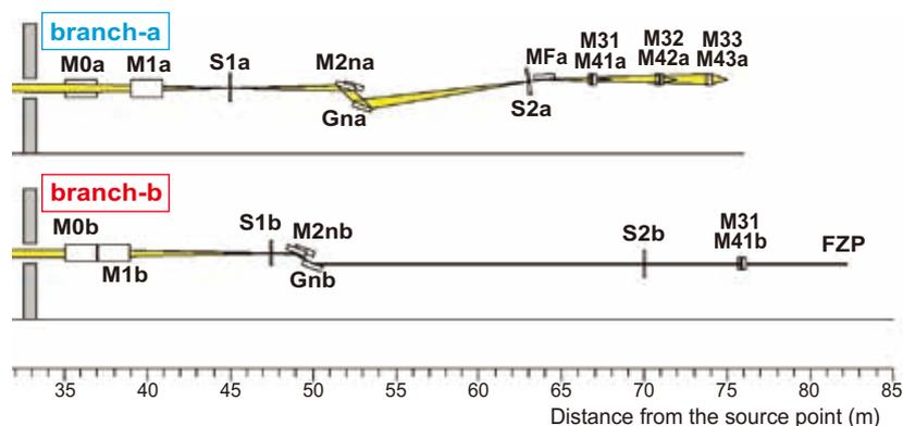
Fig. 2. Optical layout (side view) of upgraded BL25SU.
