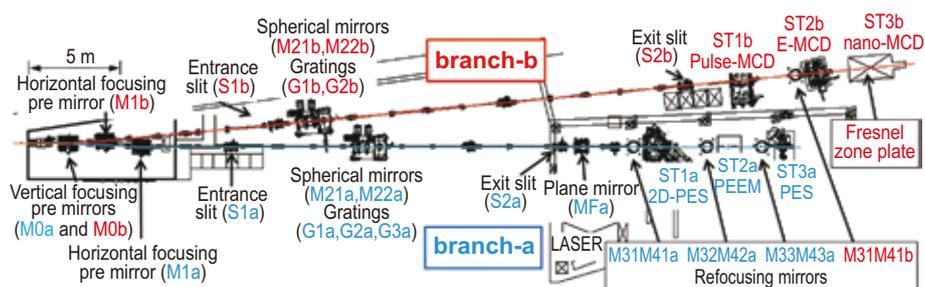
Fig. 1. Photograph and schematic view of upgraded BL25SU.
