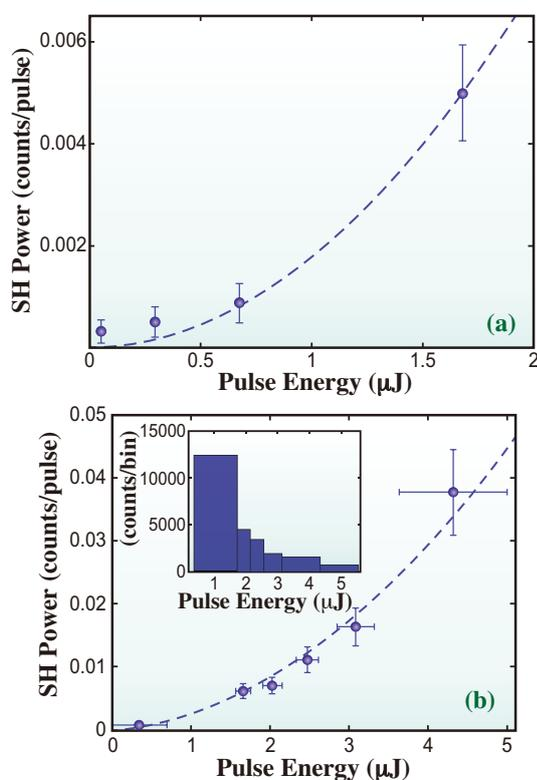
Fig. 2. Second harmonic count rate as a function of (a) Average pump pulse-energy where the pulse-energy is varied by inserting thin Al filters before the diamond crystal (b) The pulse-energy dependence is obtained from the pulse-energy fluctuations of the XFEL beam. The inset shows the energy fluctuations of the XFEL beam.
