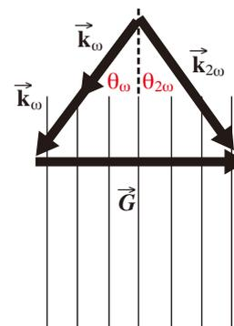
Fig 1. Phase matching diagram.
