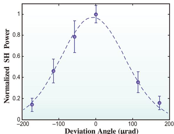
Fig. 3. Rocking curve of the second harmonic signal.
