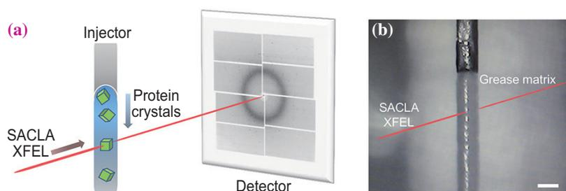
Fig. 1. Serial femtosecond crystallography. (a) Fresh nano/microcrystals are supplied for subsequent X-ray pulses to continue data acquisition. (b) Sample extrusion of the grease matrix through a syringe needle. Grease matrix was extruded as a continuous column to intersect with the XFEL beam. Scale bar represents 240  $\mu\text{m}$ .
