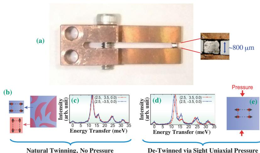
Fig. 1. Detwinning of a SrFe<sub>2</sub>As<sub>2</sub> single crystal. The top panel, (a), shows the sample glued in a holder used to exert slight pressure on the sample. The bottom panel shows the phonon response for a crystal without pressure (c) and detwinned (d). Panels (b) and (e) schematically indicate the domain structure. For (c) and (d), the sample was held at 140K <  $T_N = 200$  K.
