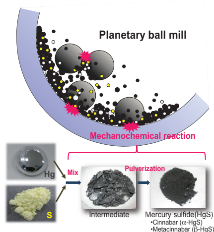
Fig. 1. Stabilization process by which elemental mercury and powder sulfur are converted to mercury sulfide by a planetary ball mill.
