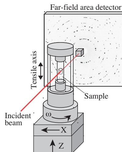
Fig. 1. Schematic of scanning 3DXRD microscopy setup.
