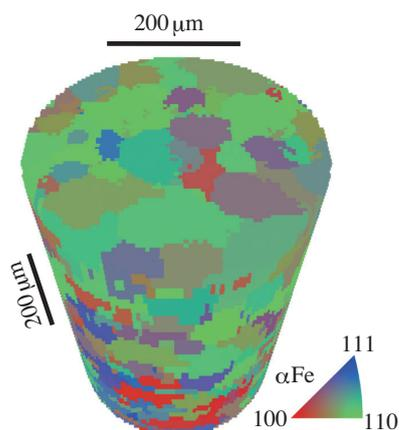
Fig. 2. 3D orientation map of coarse-grained polycrystalline iron. The colors correspond to the inverse pole figure in the tensile direction.
