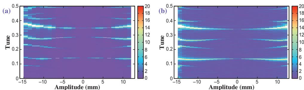
Fig. 2. Same as Fig. 1 but after optimizing the sextupole magnetic fields.
