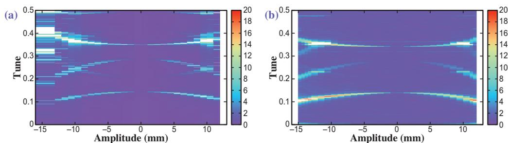
Fig. 1. Dependence of the vertical tune on the horizontal amplitude before optimizing the sextupole magnetic fields. Simulation results (a) are compared with experimental data (b).
