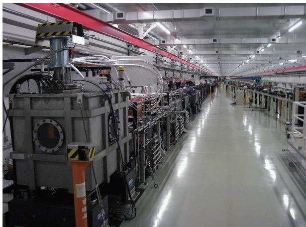
Fig. 3. Linear accelerator system dedicated to the BL1 beamline. This picture was taken from the electron gun side (i.e., the uppermost-stream side of BL1).
