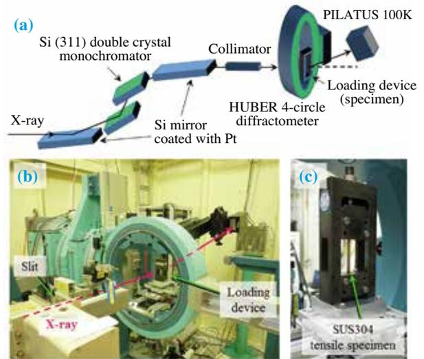
Fig. 1. Instruments for *in situ* measurement of X-ray diffraction data under stress. (a) Schematic illustration of experimental layout. Photographs of (b) 4-axis diffractometer at BL02B1 and (c) SUS304 tensile specimen mounted on a loading device.
