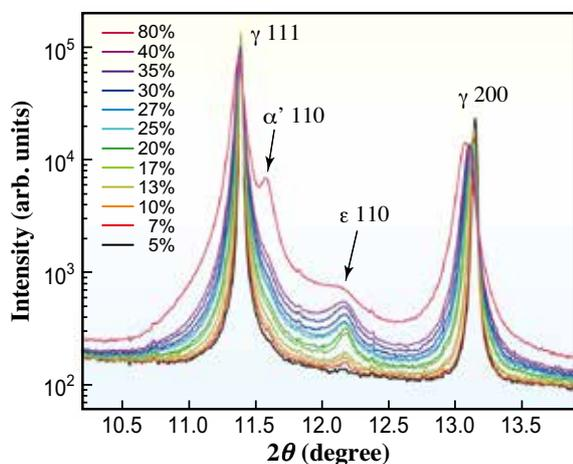
Fig. 2. Evolution of X-ray diffraction patterns in *in situ* measurement under stress. The percentages indicate the elongation applied to the specimen.
