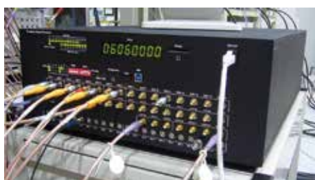
Fig. 1. New digital feedback processor for the BBF system.
