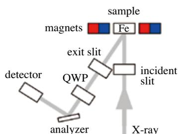
Fig. 2. Top view of the experimental layout. QWP: diamond phase retarder that acts as a quarter-wave plate. Analyzer: Ge(400) single crystal that is used as both an energy and polarization analyzer.
