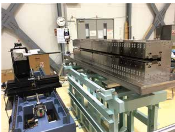
Fig. 1. Permanent dipole magnet under magnetic field measurement. The magnet consists of four segments; the first and third segments are made of samarium-cobalt, and the second and fourth segments are made of neodymium-iron-boron (NdFeB).
