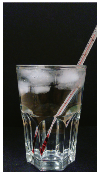
Fig. 1. A glass of ice water with a thermometer measuring 4 degrees C at the bottom.
