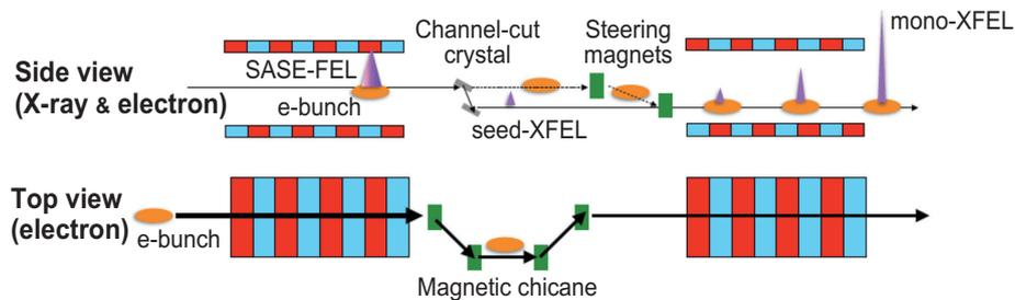
Fig. 1. Schematic drawings of the reflection self-seeding scheme.
