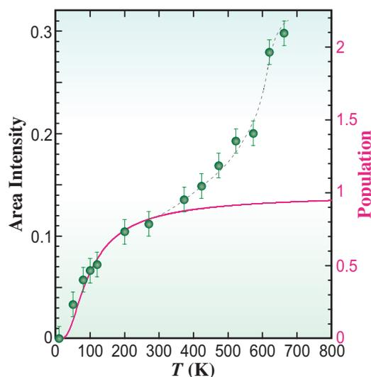
Fig. 3. Temperature dependence of the area intensity of the difference Compton profiles.
