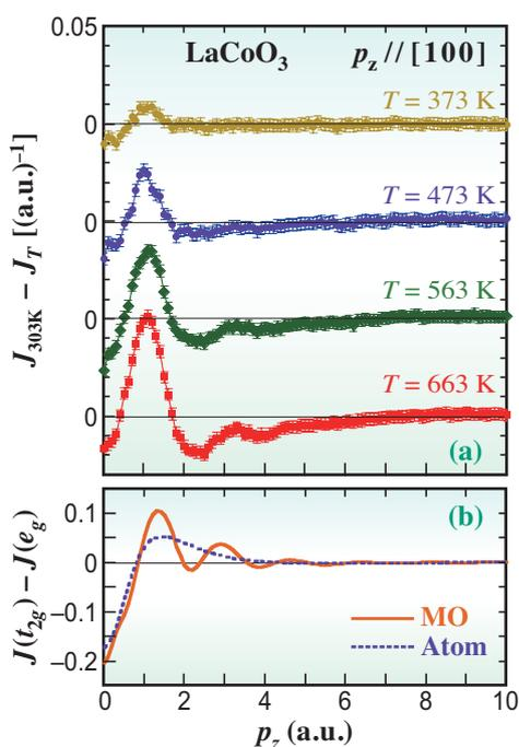
Fig. 2. (a) Temperature dependence of the difference Compton profiles ( $J_{303 \text{ K}} - J_T$ ;  $T = 373 - 663 \text{ K}$ ) for  $[100]_c$  direction of the pseudocubic unit cell, along with (b) the calculated difference Compton profiles for molecular orbitals (MO) and localized atomic orbitals (Atom).
