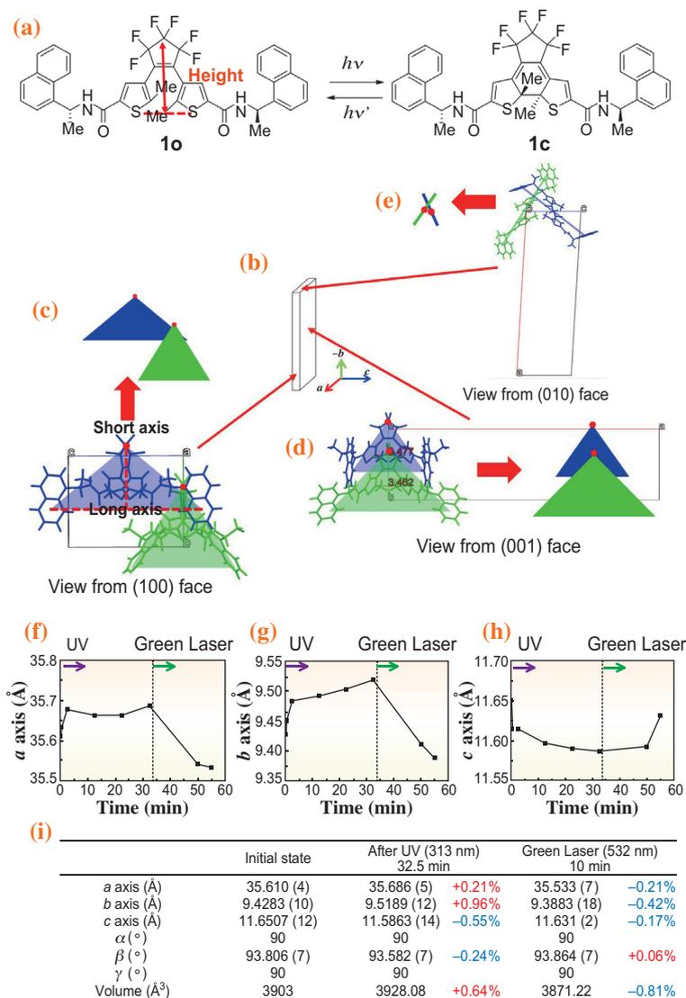
Fig. 1. Molecular packing of diarylethene **1o** in the crystal prepared by sublimation, and the size changes of the unit cell upon alternate irradiation with UV and visible light. (a) Molecular structural changes of diarylethene **1o**, (b-e) molecular packing of two conformers (illustrated with green and blue triangles) of **1o** in the unit cell, (f-i) size changes of unit cell of **1o** upon alternate irradiation with UV and visible light.
