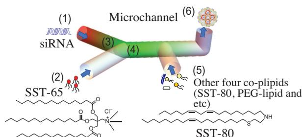
**Fig. 2.** Schematic illustration of the two-step mixing microchannel and chemical structures of SST-65 and SST-80. The numbers in parentheses show the lipoplex components (and mixing process).
