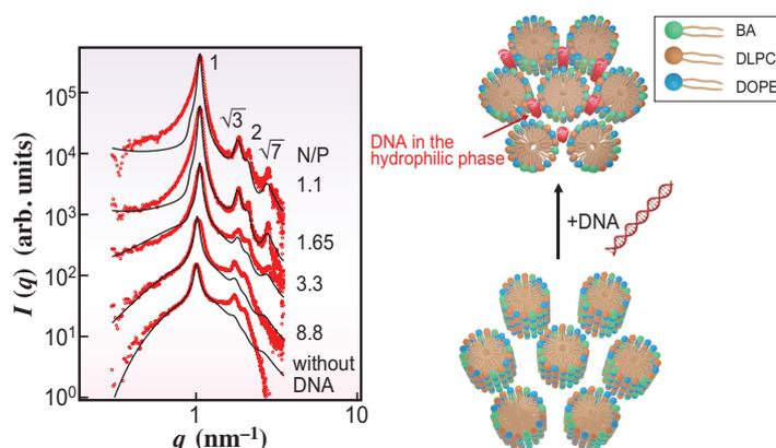
Fig. 1. N/P ratio dependence of SAXS profiles at composition B and schematic illustration of structural transition of the complex by adding DNA. Red dots and black lines show experimental data and theoretical curves, respectively.
