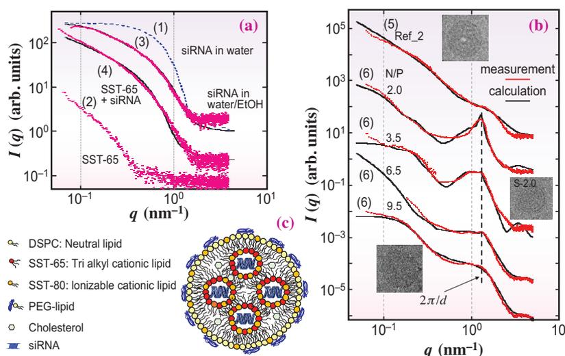
**Fig.3.** (a) SAXS profile changes on adding SST-65 to siRNA, (b) SAXS profiles at different N/P samples as well as TEM images. Red dots and black lines show experimental data and theoretical curves, respectively. The numbers in parentheses in (a) and (b) show the corresponding scattering profiles with the lipoplex components shown in Fig. 2. (c) Schematic illustration of the lipoplex. [5]
