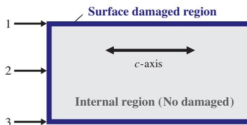
Fig. 1. Schematic illustration of the depth-dependent measurement of SSMH for the neodymium magnet.
