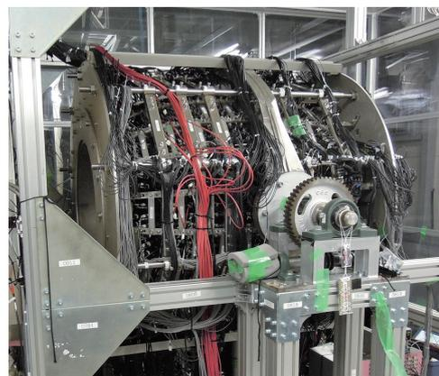
Fig.1. Photograph of the BGOegg calorimeter, assembled with 1320 BGO crystals.
