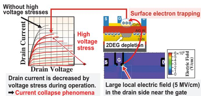
Fig. 1. Schematic of current collapse phenomenon in GaN-HEMT, originating from surface electron trapping.
