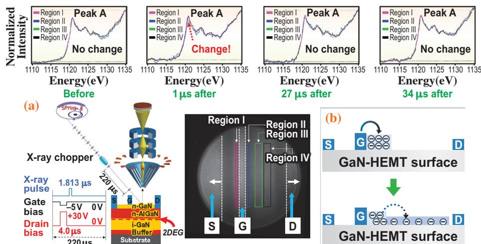
Fig. 2. (a) Spatiotemporal observation of surface electron trapping in GaN-HEMT using spatiotemporal *operando* X-ray absorption spectroscopy and schematics of the experimental system. (b) Proposed mechanism of surface electron trapping based on results of DC *operando* X-ray photoelectron microscopy and spatiotemporal *operando* X-ray absorption spectroscopy. S, G, and D indicate the source, gate, and drain electrodes, respectively.
