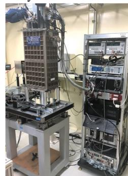
Fig.1. (a) Spectra of SRM610 taken with TES (red) and SDD (blue). (b) Experimental setup of TES system in BL37XU.
