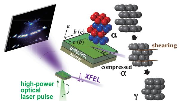
Fig. 1. Experimental setup at SACLA BL3 for analyzing time evolution of forsterite structure under compression, and the observed transformation process.
