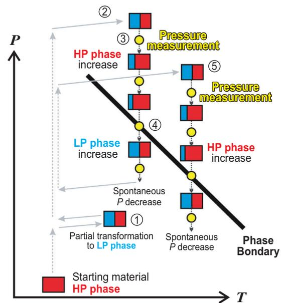
Fig. 1. Experimental strategy. The pressure spontaneously and gradually decreases while keeping the temperature and press load constant. In the high-pressure (HP) and low-pressure (LP) phase stability fields, the HP and LP phases increase with time to bracket the phase boundary. The numbers in the circles indicate the step numbers in the new strategy explained above.
