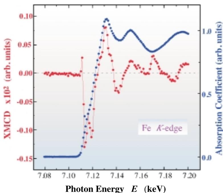
Fig. 3: XMCD spectrum at the Fe *K* edge in Fe<sub>4</sub>N recorded by the helicity-modulation technique. The normalized XANES spectrum is also displayed.
