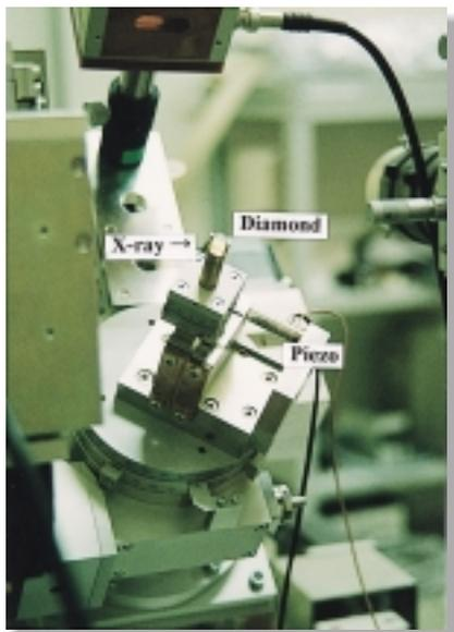
Fig.1: Assembly of the phase retarder. The diamond phase plate is fixed in a piezo-driven stage mounted on a 2-circle goniometer.
