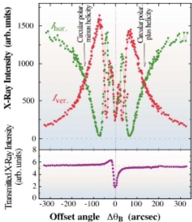
Fig. 2: Measured variations of X-ray intensities versus the offset angle with respect to the Bragg angle in the energy range of 8 keV. The vertical component is equal to the horizontal one at  $\pm 140$  arcseconds, where the polarization state of the transmitted X-ray is converted into circular polarization. The phase retarder can also function as a  $\lambda/2$ -phase plate, that is, the polarization plane is rotated from horizontal to vertical at around  $\pm 70$  arcseconds.
